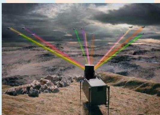
According to IAI, Scorpius' AESA's multi-beam capability allows the system to “simultaneously scan the entire surrounding region for targets, and deploy narrowly focused beams to interfere with multiple threats across the electromagnetic spectrum.” Scorpius can effectively disrupt radar and electronic sensors, navigation, and data communications, the company said.
