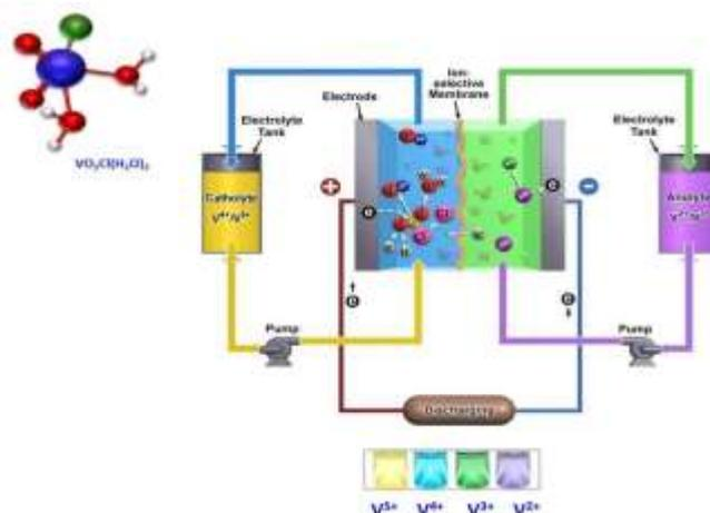
V can exist as several ions of different charges in solution,  $V(2+,3+,4+,5+)$ , each having different numbers of electrons around the nucleus (see figure). Fewer electrons gives a higher positive charge. Energy is stored by providing electrons making  $V(2+,3+)$ , and energy is released by losing electrons to form  $V(4+,5+)$ .
