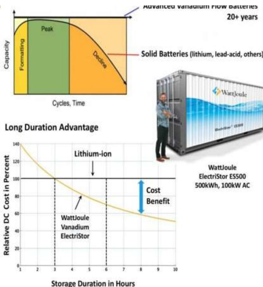
Unlike solid batteries, like lithium-ion or lead-acid, that begin degrading after a couple of years.
