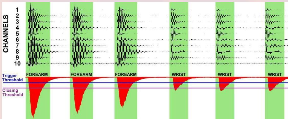
Figure 6: Ten channels of acoustic data generated by three finger taps on the forearm, followed by three taps on the wrist. The exponential average of the channels is shown in red. Segmented input windows are highlighted in green. Note how different sensing elements are actuated by the two locations.
