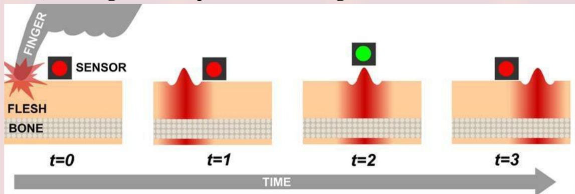
Figure 2. Transverse wave propagation: Finger impacts displace the skin, creating transverse waves
