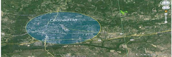
In dynamic geofencing the information regarding restricted area is continuously propagated. Static geofencing uses a flight permission information repository, which when accessed by the intruding drone denies it access beyond the intended point.Most commercial drones use internal auto-landing modules for safety. Geofencing is unable to disable these automatic landing systems.
